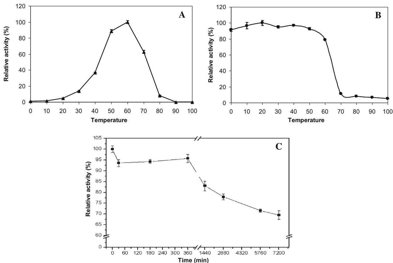
**Fig. 3.** Effect of temperature on catalytic activity. (A) The optimal temperature was determined under standard assay conditions. (B) The temperature stability was determined by measuring the remaining activity after incubation at various temperatures at pH 6.0 for 30 min without substrate. (C) The remaining activities after incubation at 50 °C without substrate at various time points were reported.
